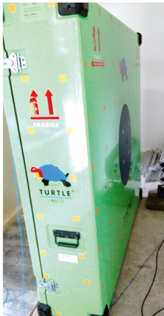
9. - 10. Measuring points on the TURTLE uNLtd and on the wooden climatic crate for the experimental modal analysis.
