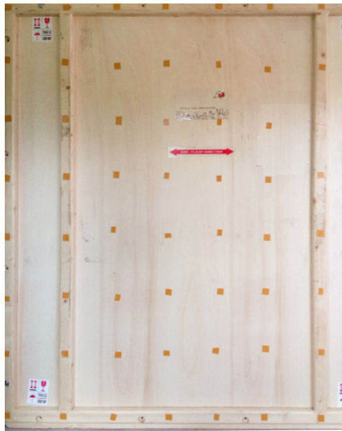
9. - 10. Measuring points on the TURTLE uNLtd and on the wooden climatic crate for the experimental modal analysis.
